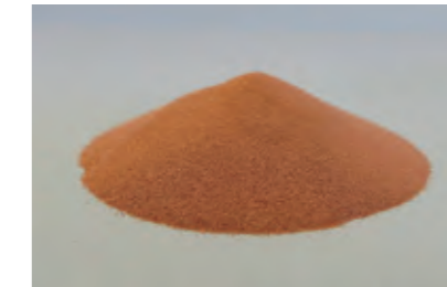
Pure copper powder used for metal additive manufacturing with surface treatment
