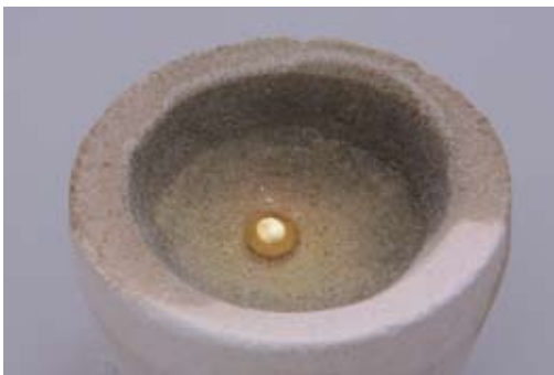
Gold bead obtained by fire assay analysis method
