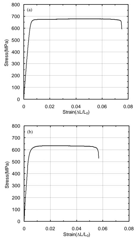
Fig.7 Stress-Strain curves for NKC164-H in the (a)longitudinal and (b)transverse directions.
