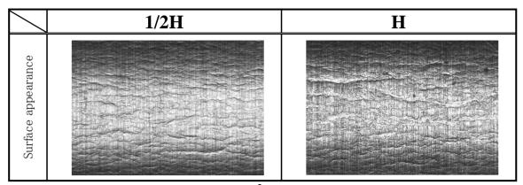
Fig.5 Surface appearances of 90° W-shaped bending test specimens(R/t=1.0). Thickness = 0.20mm, Width =10mm, Good Way
