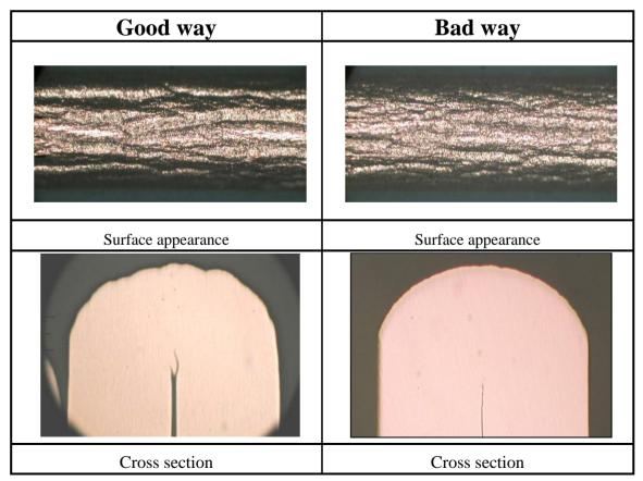
Fig.2 Surface appearances and cross sections of U-shaped bending test specimens. Temper H , Thickness = 0.25mm , R/t=0 , Width =10mm
