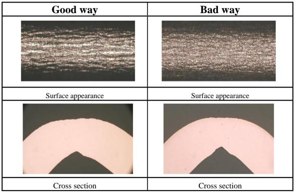
Fig.1 Surface appearances and cross sections of 90° W-shaped bending test specimens. Temper H , Thickness = 0.25mm , R/t=0 , Width =10mm
