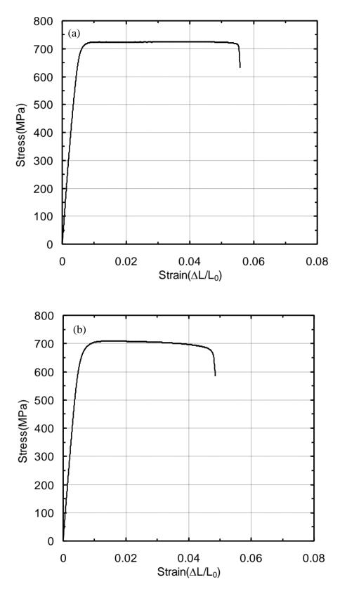
Fig.8 Stress-Strain curves for NKC164-EH in the (a)longitudinal and (b)transverse directions.
