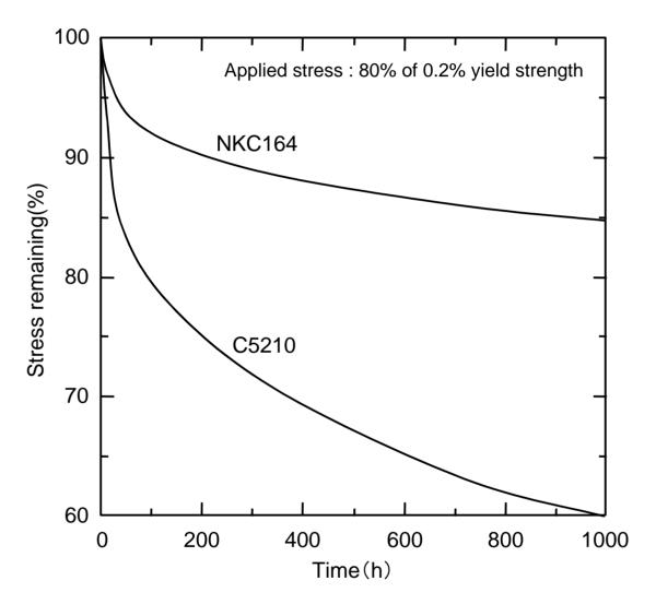
Fig.6 Stress relaxation of connector alloys at 150°C.
