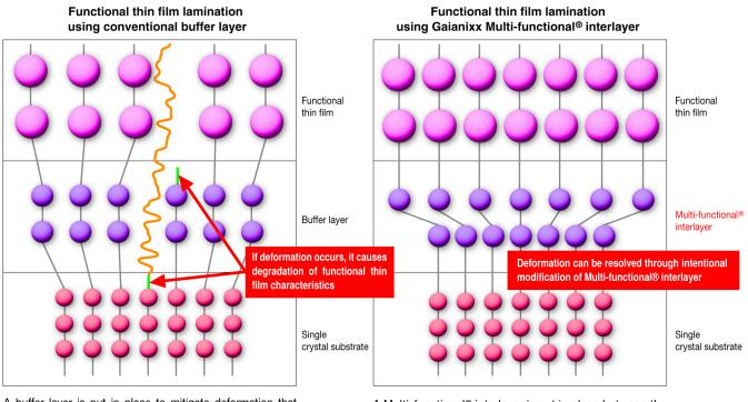
A buffer layer is put in place to mitigate deformation that occurs from mismatch in the lattice constant (length of crystal axis and angle between axes) of the single crystal substrate and the functional thin film.
