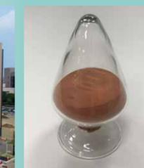
Pure copper powder for additive manufacturing
