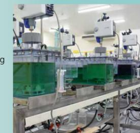
Bench scale equipment for EV lithium battery recycling
