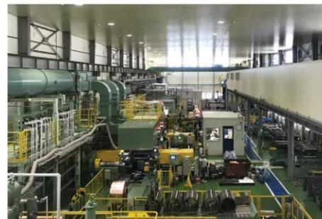
Manufacturing equipment for treated rolled copper foils and advanced copper alloy (Kurami Works)
