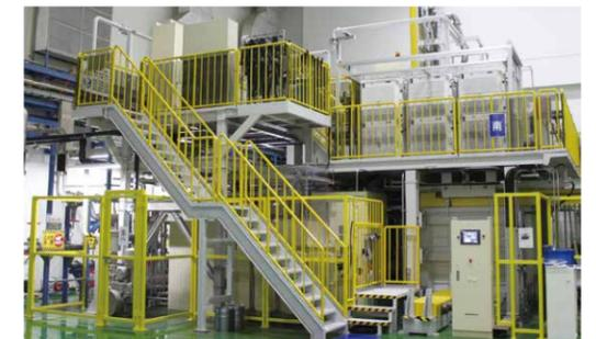
Melting furnaces, equipment used for semiconductor-use sputtering targets (Isohara Works)
