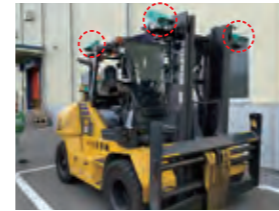
Cameras installed on forklifts
