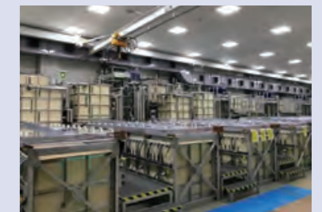
Production equipment used for semiconductor-grade sputtering targets such as electrolysis baths (Ishihara Works)
