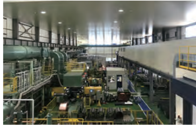
Rolling mills for treated rolled copper foil and high-performance copper alloys (Kurami Works)
