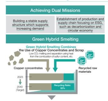
We offer copper products using Green Hybrid Smelting. Both copper concentrates and scrap can be used as raw materials. The heat generated by the copper concentrates itself can be used to melt recycled materials, making fossil fuels virtually unnecessary.
